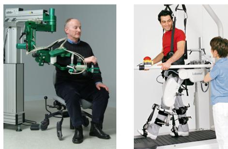
**Figure 1** ARMin and Lokomat upper and lower extremity exoskeletons (Lokomat photo courtesy of Hocoma AG, Switzerland).
